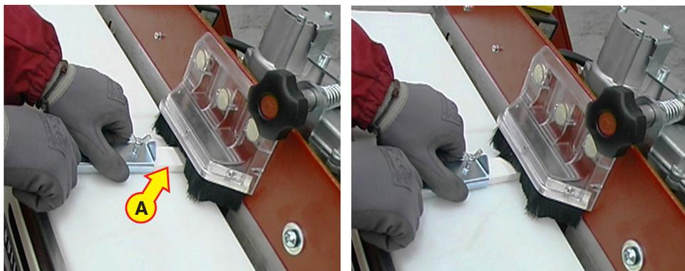
Position the spray guard so that the brushes are in contact with the carriage table. Turn the machine on and wait for cooling water to reach the grinding wheel. Insert the sharpening stone in the stone holder. Hold the sharpening stone (A) against the grinding wheel. Hold it down whilst turning it alternately rightwards and leftwards. This operation must be repeated until the grinding wheel is sharp again.
