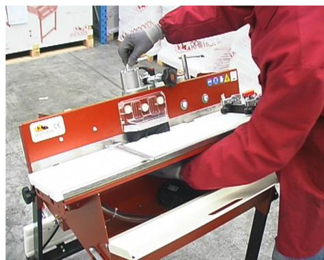
Using a size 30 wrench (C), undo the grinding wheel fixing nut (D) by turning it clockwise. Fit the new grinding wheel and lock it in place by turning the nut (D) counter-clockwise. Remove the B8 hexagon wrench (E). Try turning the cutter by hand to make sure it has been correctly fitted. Refit the spray guard (A).
