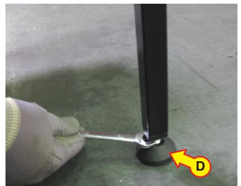
Lift the machine until the two safety bars can be inserted (B1). Lower the machine until the leg touches the safety bars (B1). Firmly screw the leg fixing knobs (C). Regulate the adjustable feet (D) to stabilize the machine.
