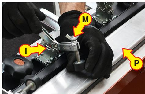
**! BEFORE STARTING PROCESSING, MAKE SURE THAT THE PRESSING DEVICE OR CLAMPS (I) DO NOT INTERFERE WITH TOOLS OR PROTECTIVE DEVICES.**
