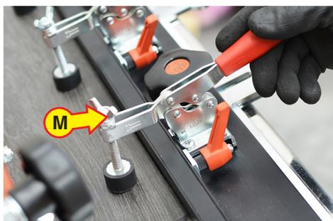
**!** BEFORE STARTING PROCESSING, MAKE SURE THAT THE PRESSING DEVICE OR CLAMPS (I) DO NOT INTERFERE WITH TOOLS OR PROTECTIVE DEVICES.
