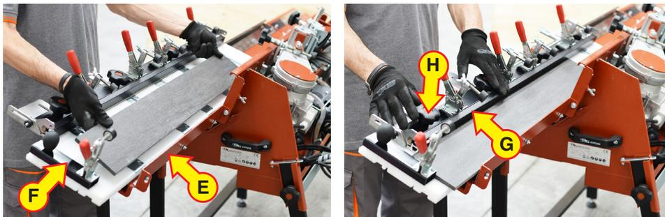
Position the material to be shaped onto the trolley perfectly rested against the frame slide (E) and against the rear support (F) of trolley. In order to prevent the material from shifting, draw the black square (G) near it and lock it by knobs (H).
