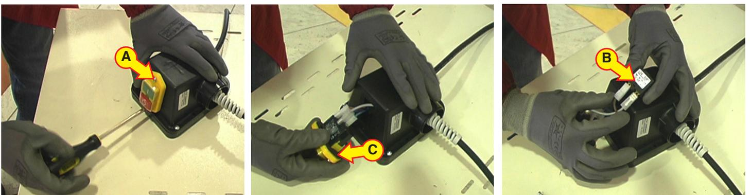
Remove the starting device unscrewing the fixing screws (A). Disconnect the electric cables and replace the on/off switch or the damaged thermal relay (B). Reconnect the cables and tighten with the previously removed screws. Make sure the seal gasket (C) is not damaged. Replace it if needed.
