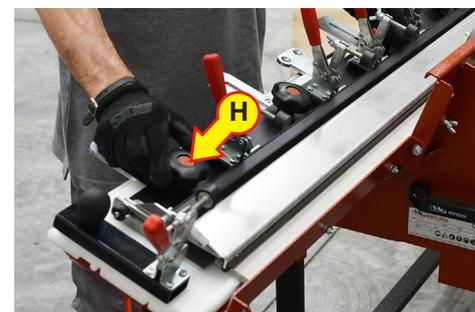
Position the material to be shaped onto the trolley perfectly rested against the frame slide (E) and against the rear support (F) of trolley. Loosen side knobs (O) and extract steel square from below the black square up to its end of stroke and tighten them. In order to prevent the material from shifting, draw the steel square (G) near it and lock it by knobs (H).
