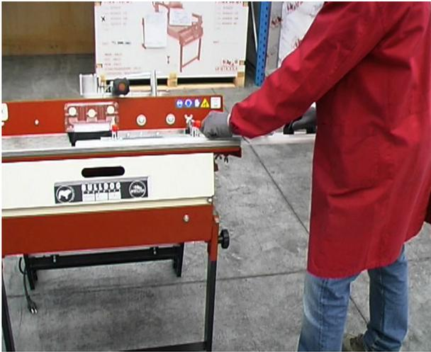
The BULLDOG ADV series shall be used by one single operator, who will have to stand sideways the machine and, by grabbing the trolley handle, will be able to make half-bullnose shapings, bevels and “jolly” (45° mitering) cuts in safe conditions and unstressfully.
