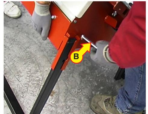
Free the front legs by completely unscrewing the leg fixing knobs (A). Go to the front side of the machine and lift it so that the leg goes past the left and right safety bars (B) and at this point close the bars.
