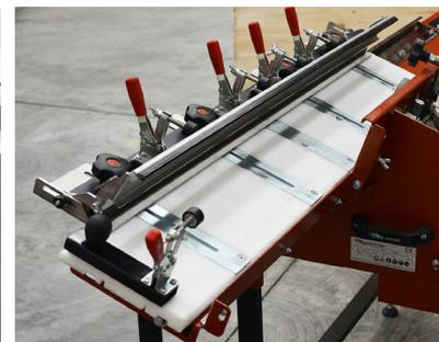
In order to use this material size, the pressing device (P) must be assembled onto side supports. Screws (Q) must be loose in order to ensure its movement. Use properly sized wrenches (R) to assemble the pressing device.
