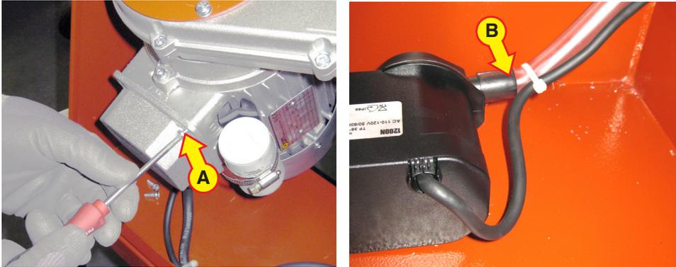
Empty the tank. Open the terminal block cover of the main electric motor (A). Unplug the pump's power supply cable. Disconnect the water delivery hoses (B). Replace the damaged pump with a new one, and restore connections. Close the terminal board cover, paying attention not to crush the wires. Reconnect the delivery hoses.
